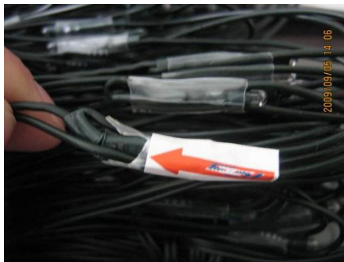
Defect: broken sleeve
