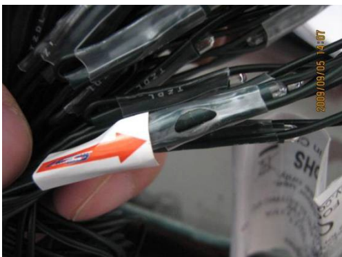
Defect: broken sleeve
