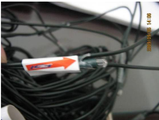
Defect: broken sleeve
